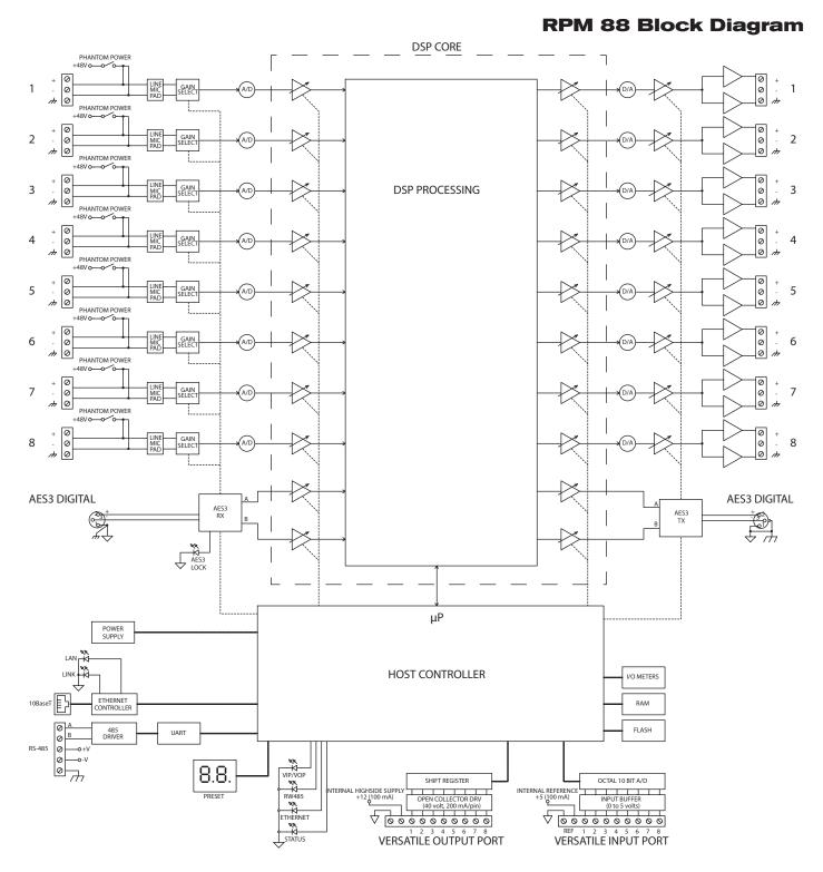
The RPM 44 uses the same Block Diagram, with four analog inputs and four analog outputs.
