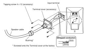
For the speaker cable, use a cable with a diameter of 6 – 10 mm, which will fit the cable bushing.
