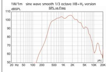
Material / Color ..... Aluminum alloy SS4263 / RAL 7031 Mounting ...... Bracket Termination ..... e-chamber, screw terminals Weight ......5,0 kg IP-rating (UL equivalent) ......67 Max / min amb temp ...... 50°C / -50°C Rated / max power ...... 20 W / 20 W 101 dB 114 dB SPL rated power ...... 117 dB 400-5000 105° / 35° Dispersion (-6dB) 1kHz / 4kHz ......125° / 35° Directivity factor, Q ..... Options ...... Impedances, colors, labels
