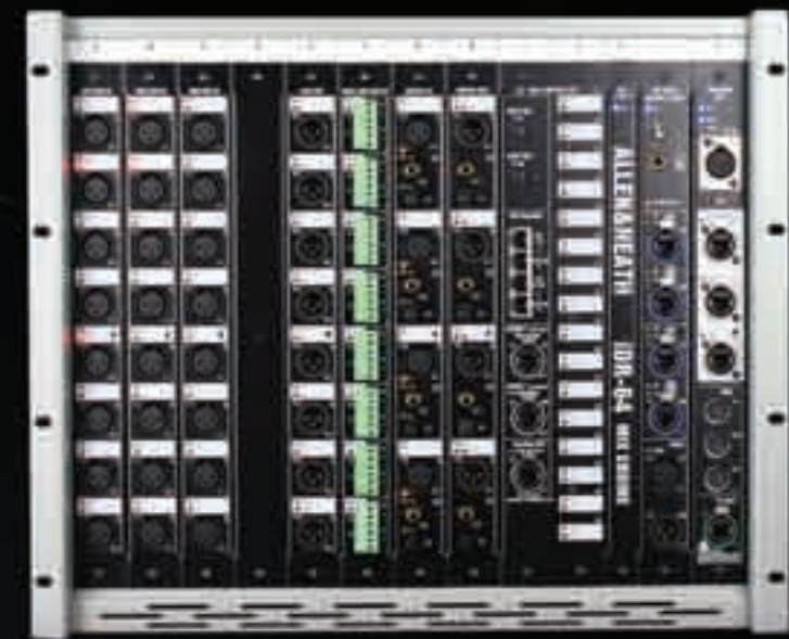
iDR10. The brain of iLive. 10 module slots for I/O in an iLive digital system along with DSP, EtherSound and control interfacing.
