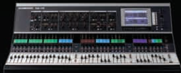
iLive-144. 144 strips arranged into 4 layers, 36 faders per layer. Makes a great choice for large concert tours.
