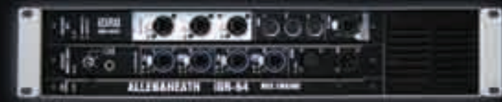
iDR0. Network mixing solution based on the DSP and CPU from the iDR10, sourcing audio by EtherSound. Ideal for mixing broadcast outputs, or splitting monitor feeds from another iLive system.
