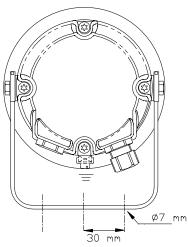
Standard model delivered with two M20 Ex approved plastic blinding plugs
